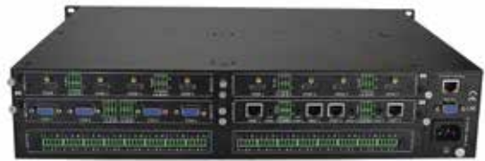
AVS800, back view, with signal cards installed
