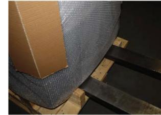
3. Gently lift away from the pallet, making sure the cabinet is properly balanced on the forks.
