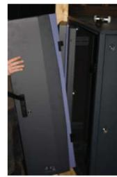
*CAUTION: Make sure the doors and side panels are placed against a solid wall on a clean, even surface after removing them from the cabinet.*
